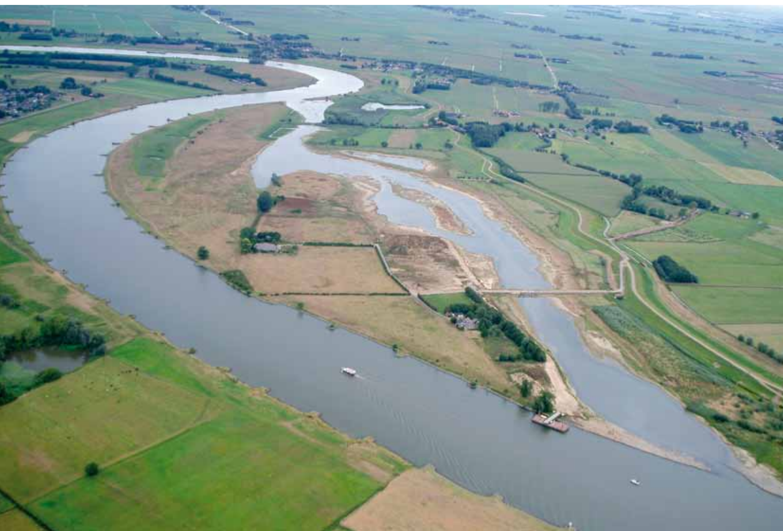
Figure 2: Redynamisation of a waterway through connection of a river branch at Vreugderijkerwaard, IJssel, Netherlands
