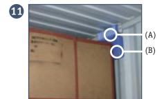
The upper part of the housing (A) contains the salt and must be exposed to the air. The lower part (B) can be covered with cargo if necessary.
