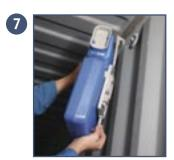
Using a stepladder and holding the bottom of the hook bar, lift the unit up all the way up to the ceiling and place the hook on the loop in the container wall.
