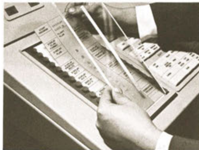
FIGURE 4: Display and Control surface of Console
