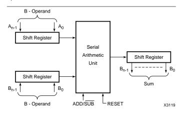
Figure 1. Serial Bit Adder/Subtracter
