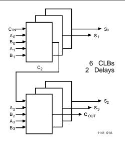
Figure 10. 4-Bit Adder
