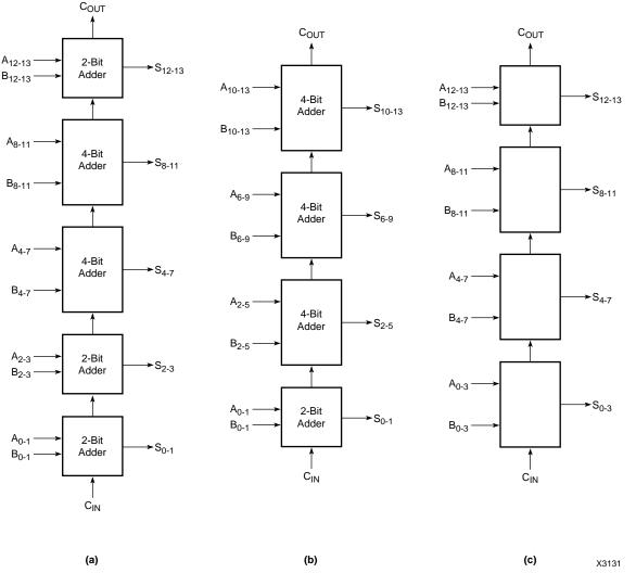
Figure 9. 14-Bit Adder Configuration
