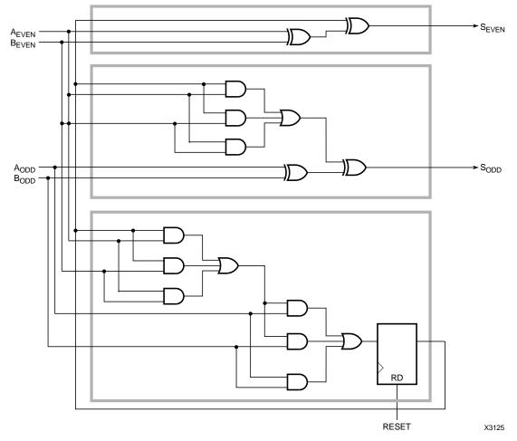
Figure 4. 2-Bit Serial Arithmetic Unit
