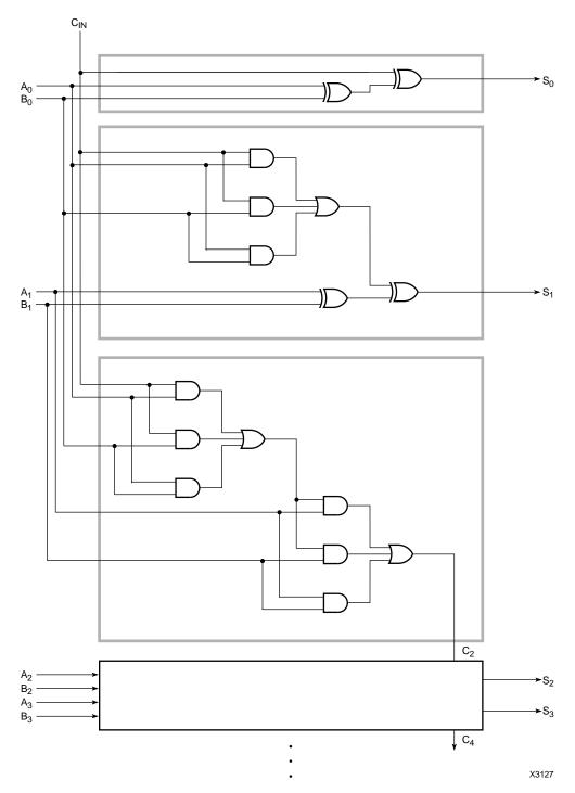
Figure 6. Two-Bits-At-A-Time Ripple-Carry Adder
