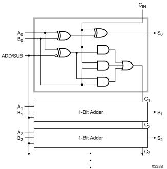
Figure 5. One-Bit-At-A-Time Ripple-Carry Adder
