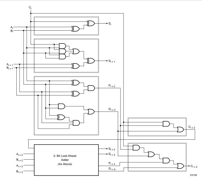
Figure 7. Four-Bits-at-a-time Adder Block with Internal Look-Ahead Carry
