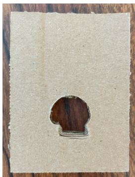
Figure 49 | 10 mm round hole tear
