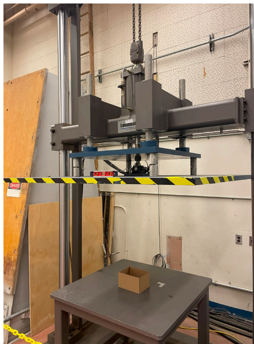
Figure 34 | Compression strength test set-up
