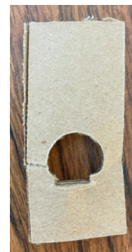
Figure 51 | 10 mm round hole, 10 mm side breakage
