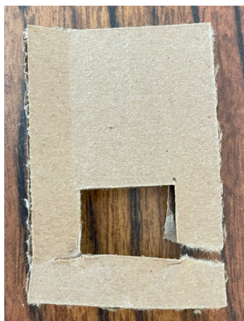
Figure 52 | 10 mm side breakage
