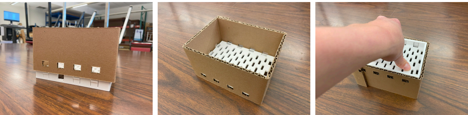
Figure 24 | Rapid prototyping of push through snap system concept (on scale)
