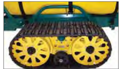
Optional Flotation Tracks smooths out the ride, floats over wet ground and greatly reduces compaction.
