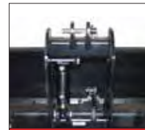
Cylinder raises scarifier beam
