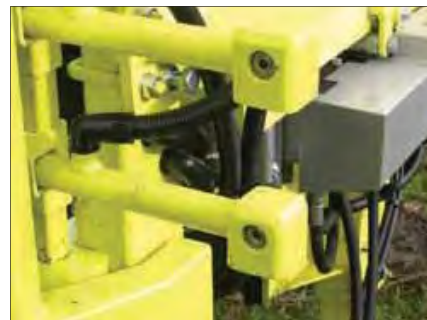
Optical cells that are for automatic opening and closing cutting heads
