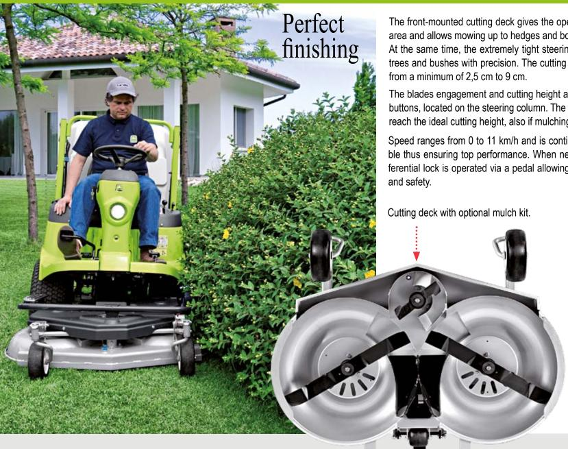
The front-mounted cutting deck gives the operator extraordinary visibility of the working area and allows mowing up to hedges and borders with high accuracy.
