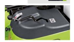
The disc parking brake is of the "active" type: once engaged, it allows you to dismount the machine with the engine running and the cutter disengaged (maximum safety).
