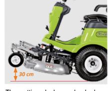
The cutting deck can be hydraulically lifted during transfer, via an electrical push-button, allowing you to traverse obstacles.
