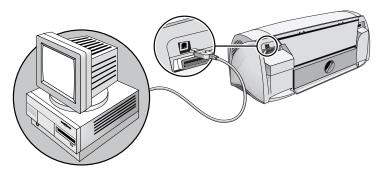
The latest personal computers have USB ports that can be directly connected to the printer's USB port. After connecting the USB cable, the **New Hardware Found Wizard** should appear. If it does not, your computer is probably not configured to use USB. Use a parallel cable instead to connect the printer to your computer.
