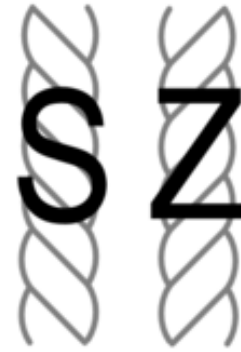
Figure 3: S Spun and Z Spun (From Wikipedia, Spinning Textiles)
