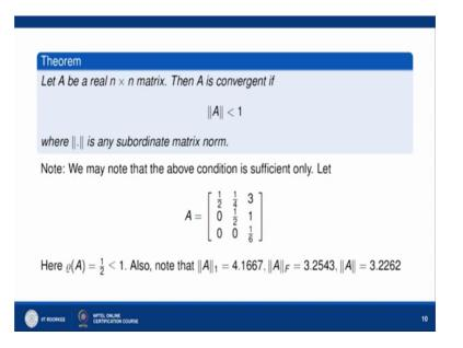
So, with the help of this result, we can define new result in terms of converging matrix. So, we say that let A be a real n cross n matrix, then is convergent if norm of A is less than one here this norm is any subordinate matrix norm. So, if you look at this is a sufficient condition because if norm of A is less than one then spectral radius of A is less than 1 and we already know that is a spectral radius is less than one implies that A is a convergent matrix..
