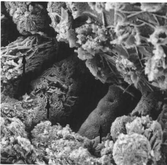
Plate 5. SEM photographs from porcellanite Sample 115-711A-20X-4, 29-37 cm. 1. Radiolarian skeleton mostly preserved as cast by opal-CT (scale bar = 40 \mu\text{m} ). 2. Detail from the surface including two radiolarian spines. The originally open center of the spines seems entirely cemented by opal-CT and only a thin coat of opal-A remained. One can easily see the bladed structure of opal-CT between the two spines (scale bar = 5 \mu\text{m} ). 3. Detail of Figure 2 (scale bar = 4 \mu\text{m} ). 4. Rim area of the radiolarian showing three spines (arrows) of different preservation stages. The right spine is still preserved as opal-A, whereas from the left spine only the opal-CT-cemented inner pore space is preserved (scale bar = 10 \mu\text{m} ). 5. Detail from the middle spine in Figure 4. Only small parts from the opal-A-composed spine wall are preserved (arrows) and most parts show opal-CT blades (scale bar = 2 \mu\text{m} ).
