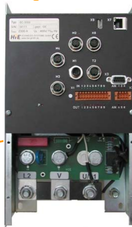
2-Phase Thyristor Module with integrated SC-3000 System Controller
