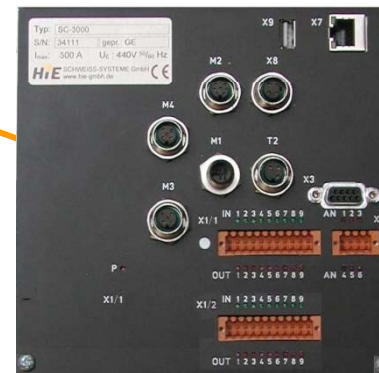
SC-3000 System Controller with extension for second welding gun
