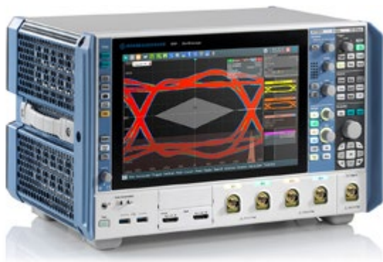
Figure 1: RTP oscilloscope. Key facts: Bandwidth 4 GHz to 8 GHz; max. sample rate: 20 Gsample/s; max. memory depth: 2 Gsample; all trigger events at full bandwidth; up to 16-bit resolution; signal integrity in realtime.
