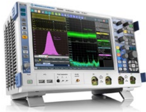
Figure 3: RTO2000 oscilloscope. Key facts: Bandwidth 600 MHz to 6 GHz; max. sample rate: 20 Gsample/s; max. memory depth: 2 Gsample; up to 16-bit vertical resolution; MSO: 16 digital channels.
