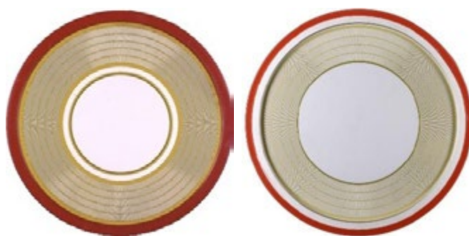
Figure 1: Left: The conventional RC-IGCT wafer with the gate contact in the separation between diode- and GCT parts. Right: The newly developed RC-IGCT wafer with the outer ring gate contact.
