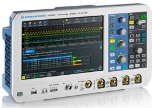
Figure 2: RTM3000 oscilloscope. Key facts: Bandwidth: 100 MHz to 1 GHz; Sample rate: up to 5 Gsample/s; Memory depth: up to 80 Msample; ADC resolution: 10-bit; Display: 10.1" capacitive touchscreen.
