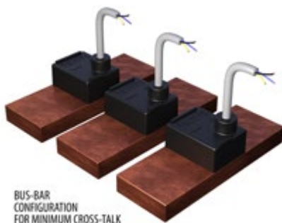
Figure 6: Simple configuration on bus-bars
