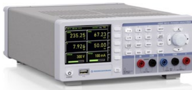
Figure 4: HMC8015 Power Analyzer. Key Facts: Power measurement range: 50 \mu W to 12 kW, analog bandwidth: DC to 100 kHz; Sampling rate: 500 ksample/s; 16 bit resolution for current and voltage; basic accuracy: 0.05 %.
