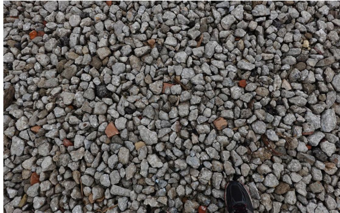
Example of processed rubble into "cultured gravel" showing bits and pieces of a variety of building material suitable as aggregate for a variety of uses.
