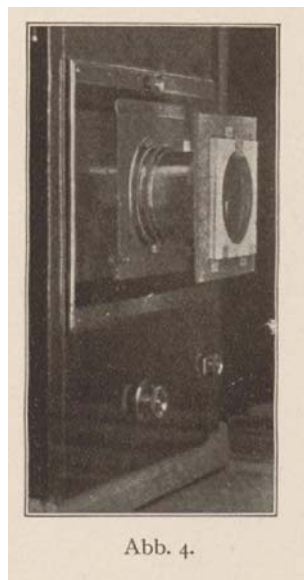
Figure 9: Glass cuvette for liquid bandpass filter positioned in front of lens.
