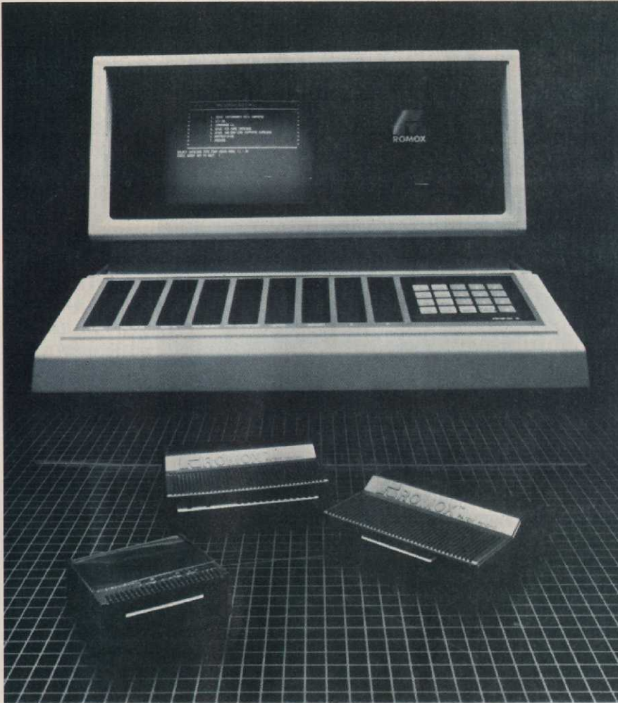
The Romox Programming Terminal allows video/computer game enthusiasts to trade in present games for the latest hits, with each terminal capable of storing 500 different titles.
