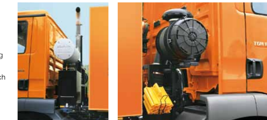
Ideal preparation for the sweeper body: lateral add-on parts such as a battery box, air intake and exhaust-gas system are situated behind the cab. As an option, the tank is mounted behind the rear axle.
