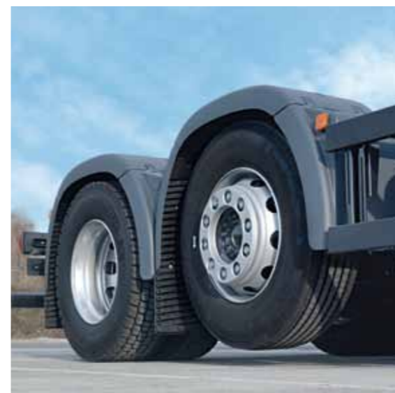
Steered, liftable leading axle on MAN TGM.
