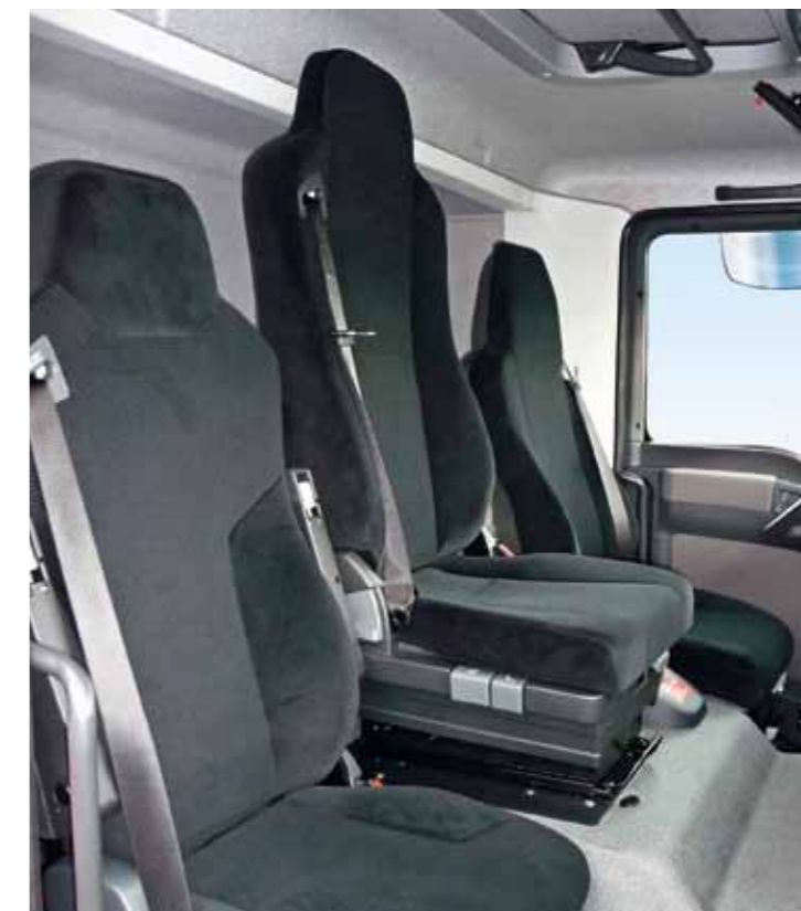
Air-sprung, adjustable center seat with integrated three-point seatbelt system.
