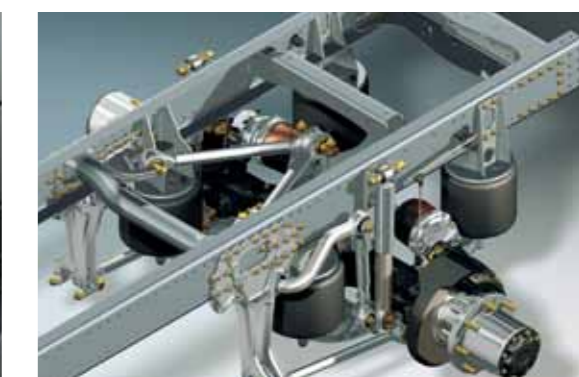
Air suspension on the rear axle of the 13-tonne vehicle.
