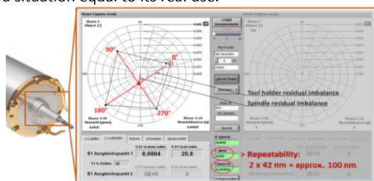
Figure 5. 3 x 90° reversal tool-holder balancing
