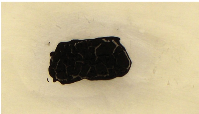
Figure 5. (a) Batteries with different amount of purified CNTs in cathodes (in fixed cells, 2640 \Omega discharge); (b) cathode cracking at high CNT percent.
