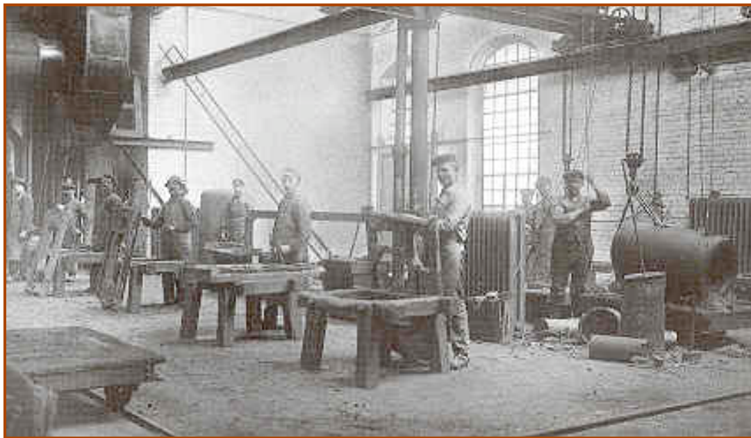
Cleaning Shop c.1928 Removing sand and unwanted ridges from the casting process
