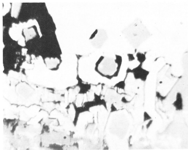
FIG. 2. Bravoite grains (dark gray) enclosed in siegenite (upper right, medium light gray), and in galena (gray). Type I zoning. Oil immersion, 550X.
