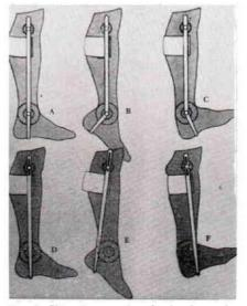
Fig. 8. This picture quite clearly shows the disadvantages of the rotation point provided on the shoe. There are shifts in vertical and horizontal directions.
