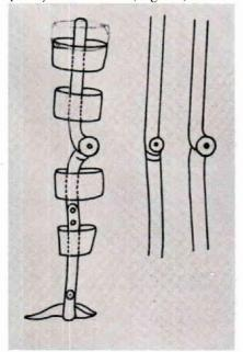
Fig. 9. Increased knee-security often sufficient in the case of partial paralysis is achieved by arranging the rotation point of the anklejoint far to the front and by the rearward location of the rotation point of the kneejoint. Schematische Dorstellung Fig. 10
