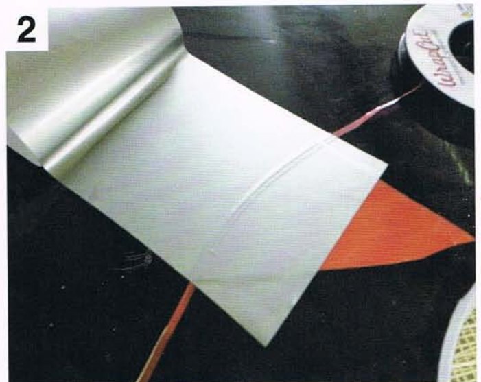
2 Stage 2 – wrap cut tape is laid along the edge of the first film with an overlap of 2mm to the thread. The second film is then laid down over the top.
