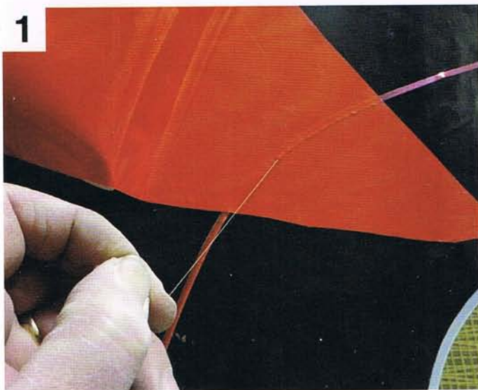
1 Stage 1 – the outline for the first colour is marked out with wrap cut tape and the first vinyl film laid on. The thread is peeled back, cutting film like a cheese wire and the tape carrier removed.
