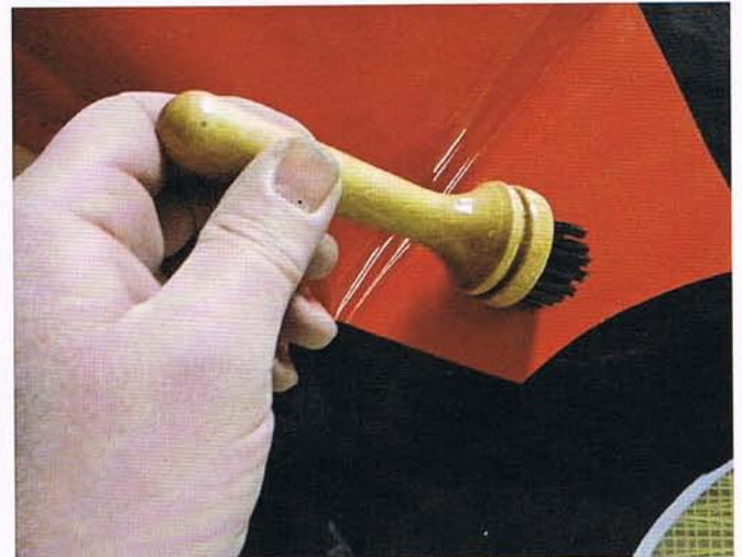
Stipple brush for ensuring all air is worked out around protrusions such as rivets.
