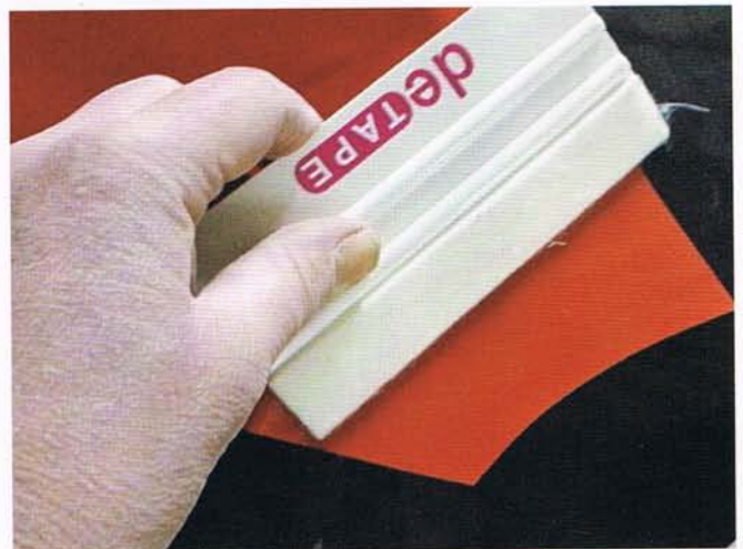
The film is heated with a hot air gun, stretched to contour and smoothed down with a felt-edged plastic squeegee, which also expels air bubbles.
