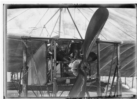
Anzani engined Blériot XI similar to the aircraft used for the Channel flight.
