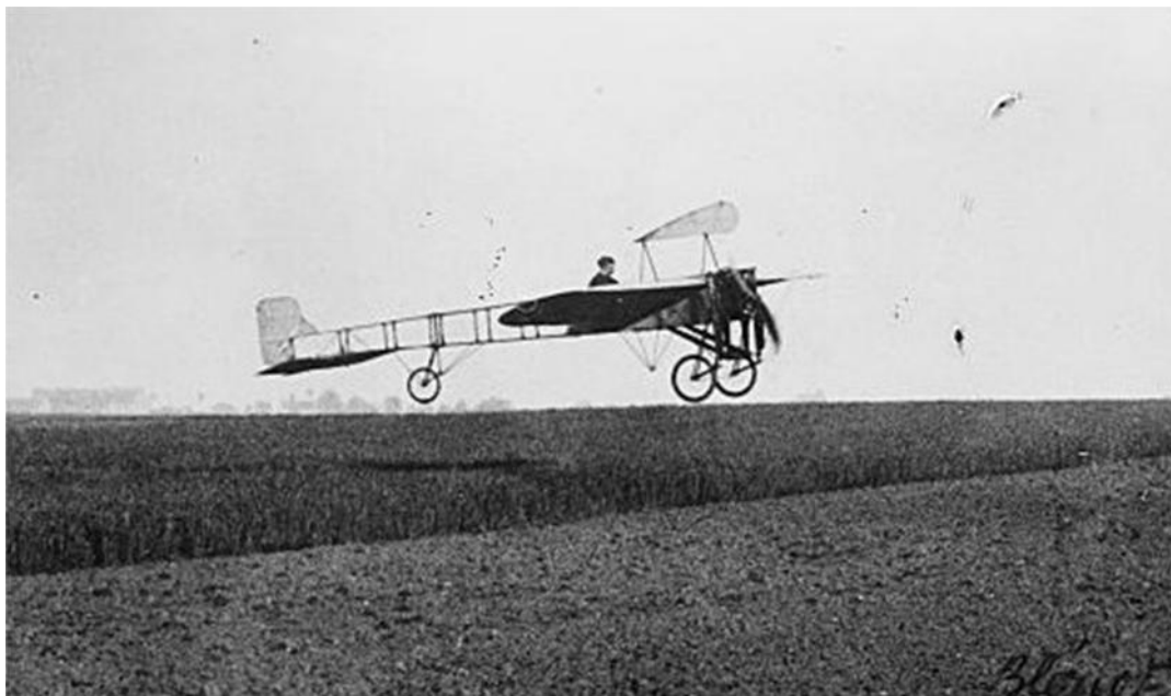
Blériot XI as first built: note small fin on cabane.
