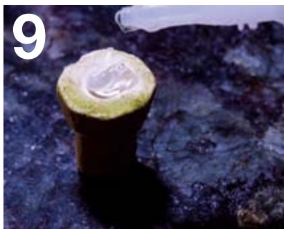
Always dry the gluing surface on the plug so the glue adheres strongly.
