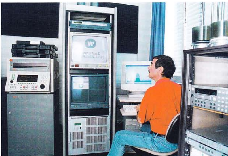
Abb. 2: BTS D1, STUDER DVD 320 Videoencoder Barco Monitore, STUDER DVD 310 Audiocoder, STUDER DVD 315 Audiocoder, (STUDER D780 DAT Recorder)
