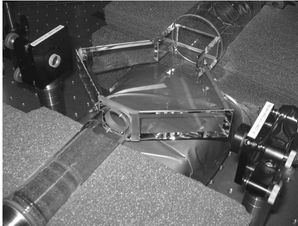
Figure 3.14: Photo of glasscell with testing resonator.
