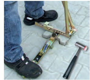
Aushebepippe AHW/ Kombihammer KH
