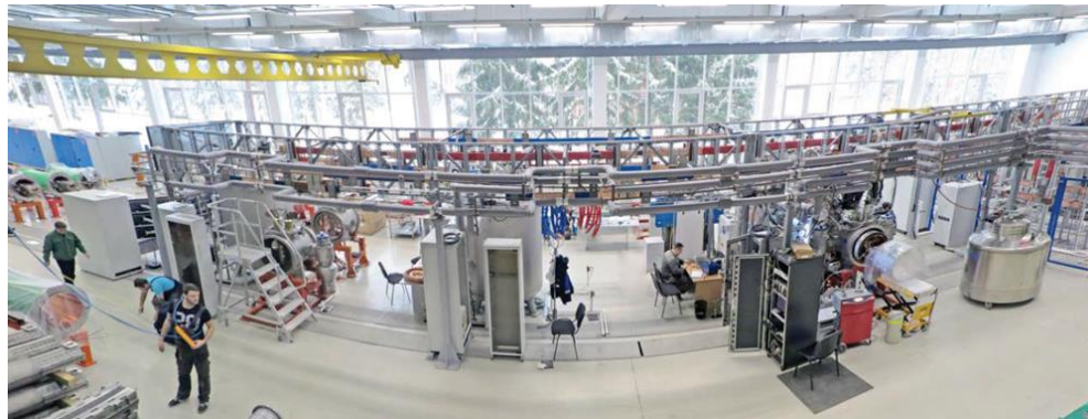
JINR, Series test facility in Dubna for testing of the series of SIS100 s.c. quadrupole units
