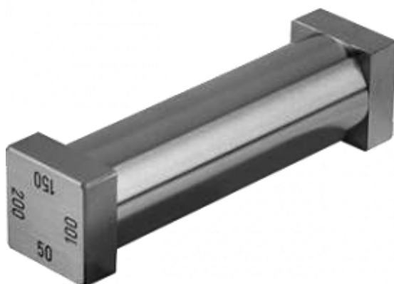
Figure 1. Applicator used to adjust film thickness
