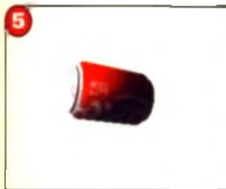
▲ Perform a scanline test render to check all is OK. A scanline render isn't as detailed as a full one, but it's faster and will include textures.
