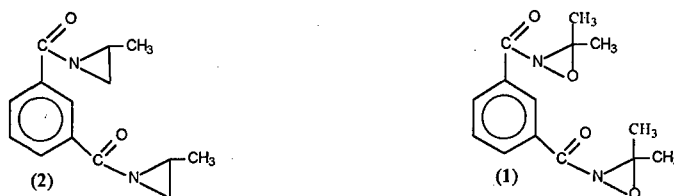
Figure 1 - Structures of Isophthalic dimethyl oxaziridine (1) and Isophthalic 2-methyl aziridine (2).
