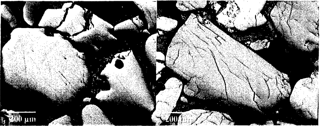
Figure 9 : Microstructure of the pressed explosive made with initial coarse grains and optimized conditions
