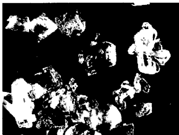
Figure 4. Micrograph of TEX. The quality of the individual TEX crystals and the favorable shape are apparent in this photomicrograph.
