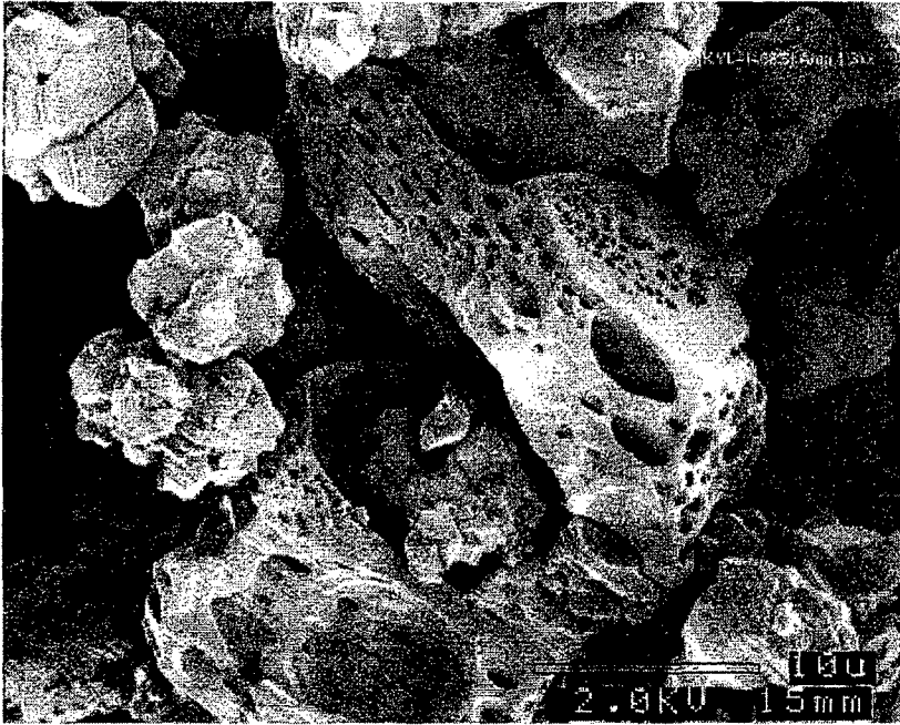
Fig. 2. SEM micrograph of FP-TATB, obtained on a Joel 6300 FXV
