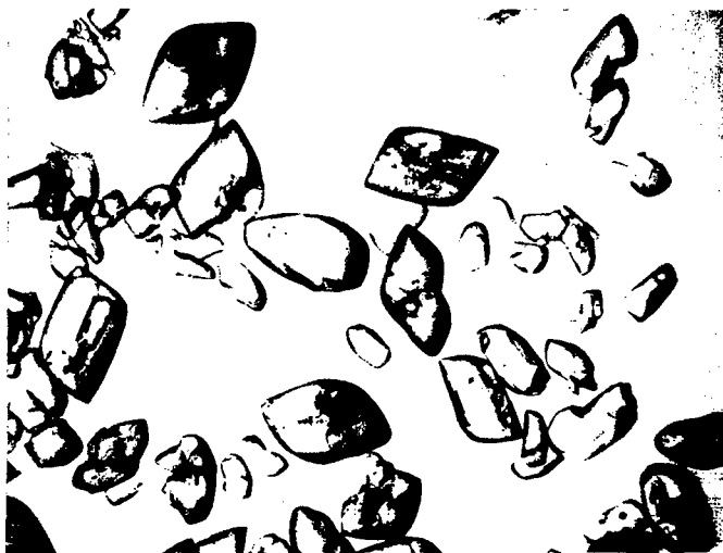
Figure 2: HMX crystals taken from the 'bad' quality batch (sieve fraction).
