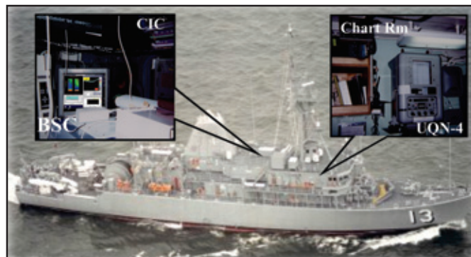
FIGURE 3 UQN-4/Bottom Sediment Classifier (BSC) installed on the USS Dextrous (MCM-13). UQN-4 fathometer display is located in the Chart Room, and the BSC display is located in the Combat Information Center (CIC) for real-time visualization of bottom type.
