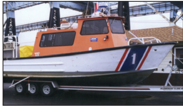
Navy range boat (30-ft, aluminum hull) coated with the NRL Fouling Release Coating System. NRL has licensed this coating system to Smart Surfaces, LLC.
