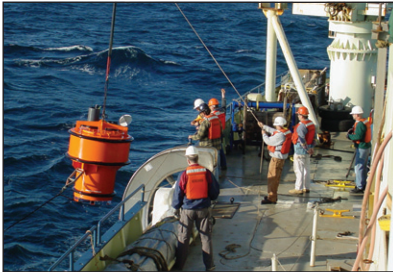
The Bottomed Vertical Line Array (BVLA) provides an autonomous system for collecting 64 channels of acoustic data for a total record time of 80 hours. The system can be controlled remotely from the ship and can telemeter data for shipboard analysis. The system can also be deployed in an L-shaped configuration, using 32-channel vertical and horizontal arrays.
