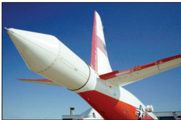
The Electra Doppler Radar (ELDORA) located on the tail and a laser mounted to the side of the fuselage of Researcher 587 were used to collect atmospheric data in the skies over Oklahoma from the International H 2 O Project (IHOP).
