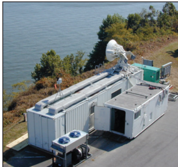
The WARLOC radar system is located at NRL's CBD. This site overlooks the Chesapeake Bay, making it ideal for research related to Naval applications. The radar system is housed in two transportable shelters. A larger shelter houses the gyro-klystron amplifier and its power supply and modulator. An integral part of this shelter is the antenna support structure that provides a rigid platform for the precision pedestal and the 6-ft Cassegrain antenna. The smaller shelter contains receivers, waveform generators, the antenna controller, and the real-time signal processing computer.
