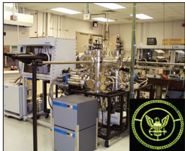
An organic, green, light-emitting diode (LED) and the advanced UHV controlled atmosphere multichamber deposition apparatus in which it was made.
