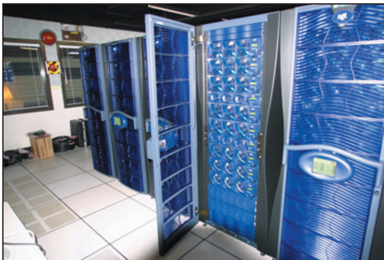
The 128-processor Silicon Graphics Origin3800 system, currently with 128 Mbytes of RAM, the first production unit in the world with R14000 processors, was brought on-line in mid FY01. The NRL Center for Computational Science, as a Distributed Center of the DOD High Performance Computing Modernization Program, provides such systems (at no cost) for anyone approved by the Program Office.
