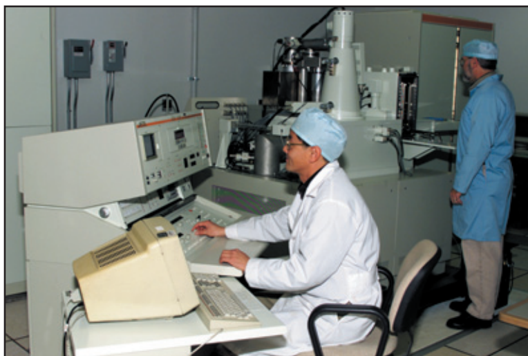
Electron beam nanowriter in use defining geometries as small as 50 Å (approximately 10 atomic layer spacings).
