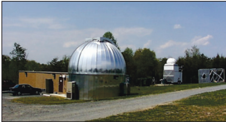
Naval Center for Space Technology Optical Test Facility at the Midway Research Center, Stafford County, Virginia. Large dome on the left houses a 1-m telescope with active laser transmit and receive capability. Smaller dome and trailer in background is a self-contained transportable 16-inch telescope that has been used as a passive optical tracker and a laser communications receiver.
