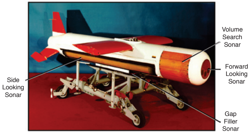
FIGURE 2 AQS-20 with the four sonars. The Volume Search Sonar is used to obtain multibeam bathymetry and sediment type.
