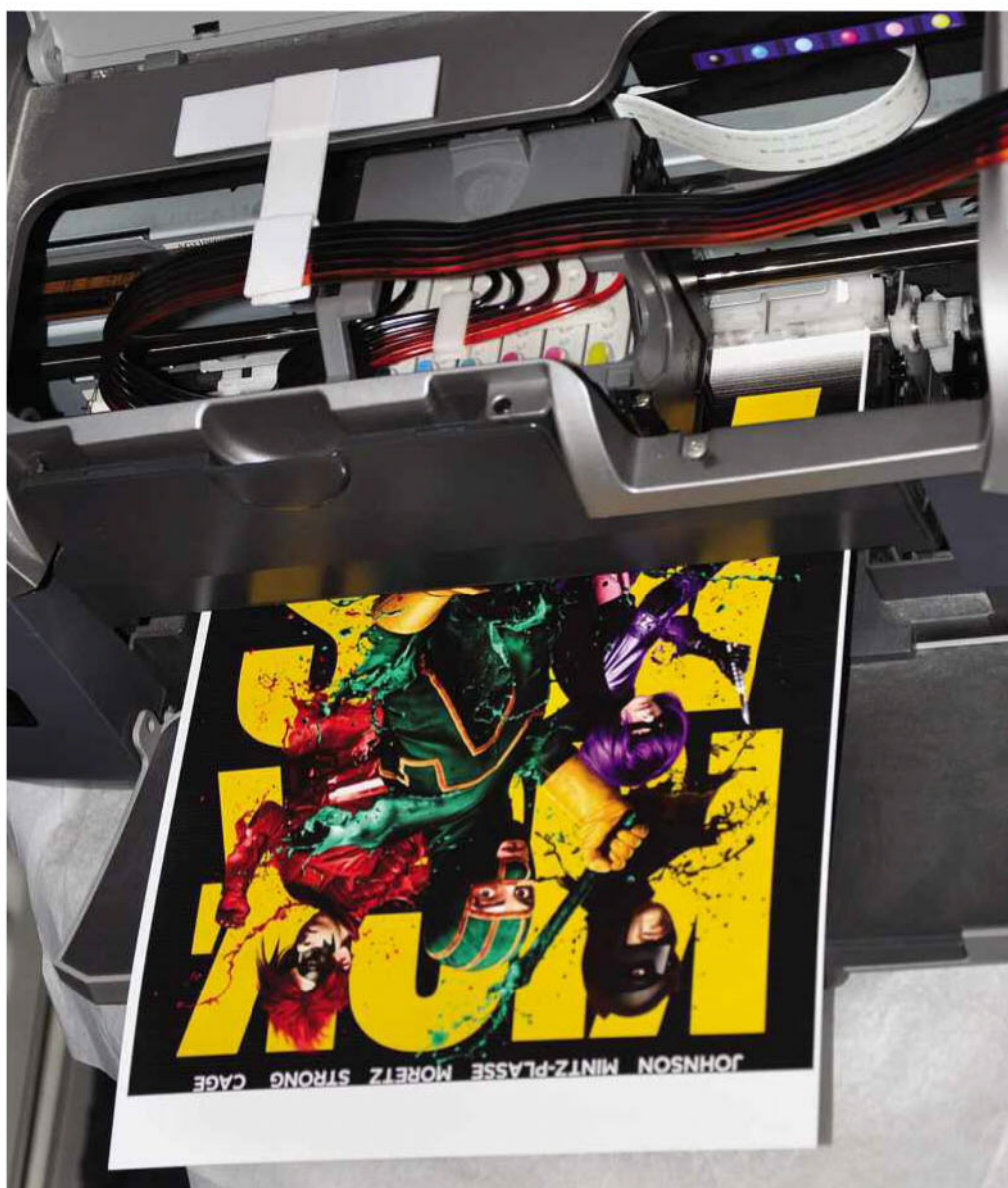
▲ A printer that has been modified with a CISS doesn't look as elegant as it once did, but it prints for much, much longer
