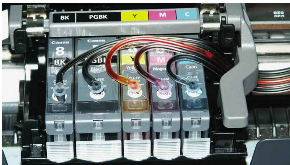
▲ Ink is pumped to a special CISS head that goes where the carts would normally be located
