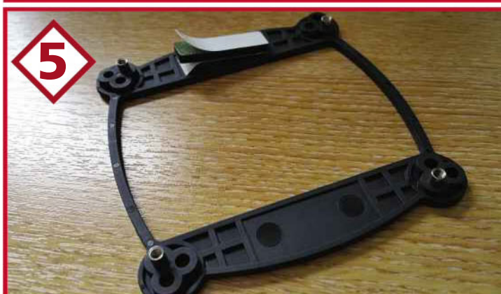
◀ Flip the backplate and apply the sticky rubber spacers
