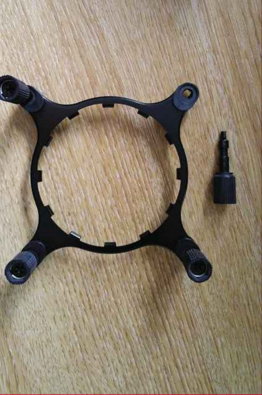
▲ The screws just push through the clips and snap into place
