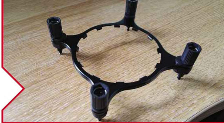
◀ With everything snapped into place, the retention ring with screws will be secure
