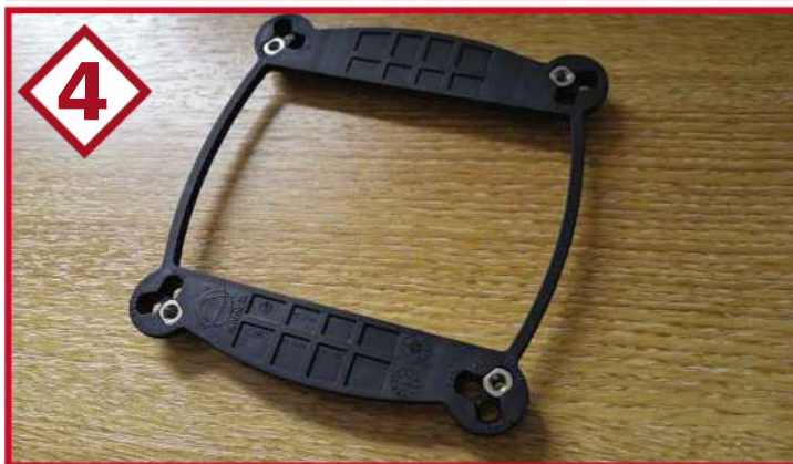
◀ The backplate, again, needs to be right one for the type of socket motherboard you have
