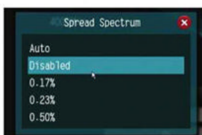
▲ With the speed set, there are a few things I want to disable. The first of these is Spread Spectrum, and the next is Speed Step. On a normal machine these features generally make the system more stable, but in this context they could create problems that I'd rather avoid. Those who feel brave can turn them back on later.
