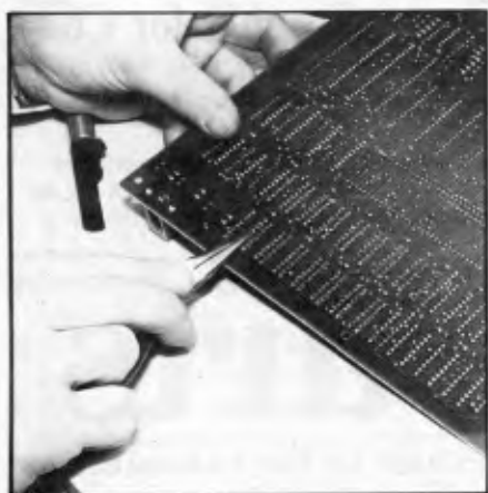
Fig 9 Straightening the IC pins
