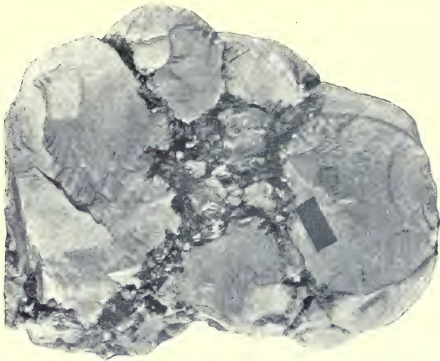
Fig. 12. Lumps of magnesite (the so-called Glockenstein). Nat. size. Bahia del Padre, Masatierra. Reproduced from P. Quensel, 12, p. 269.
