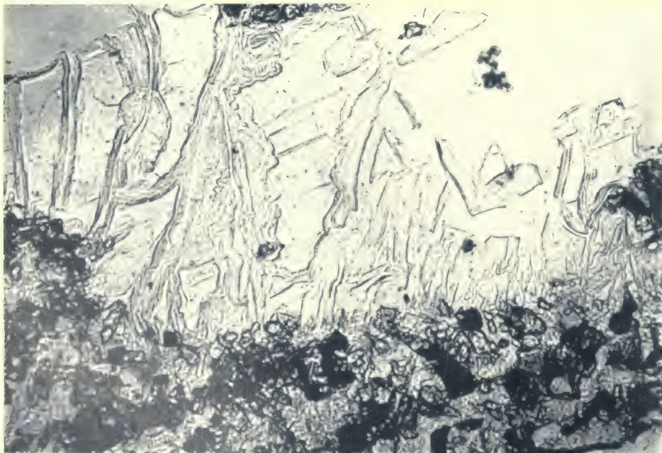
Fig. 19. Phenocryst of labradorite traversed by a zeolitic matter. \times 170 . From specimen Fig. 17. Masafuera.
