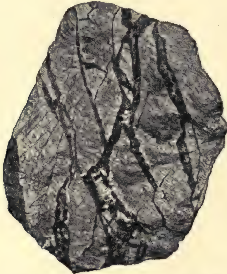
Fig. 55.—Part of a lode or compound vein (of the Traugott Spat of the Gesegnete Bergmann's Hoffnung Mine, near Oberguna) showing gray gneiss traversed by narrow stringers of galena and some quartz.
