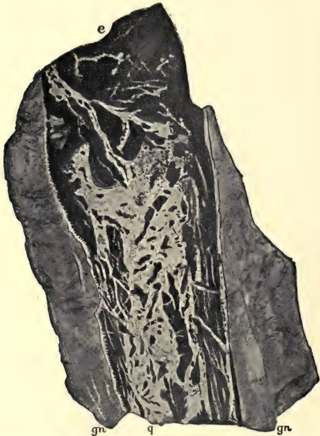
Fig. 126.—View of the vein of the Traugott Spat (rich quartz formation). From nature; an example of a vein reopened many times in succession. (Composite vein.) gn, decomposed gneiss; q, vein filling, consisting essentially of quartz; e, ore, mainly argentiferous blende, with some copper pyrite, as well as galena.
