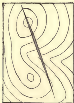
Fig. 30.—Course of the outcrop of a vertical bed in irregular topography.
