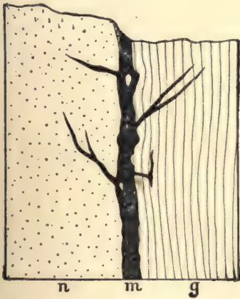
Fig. 12.—Section of a pyrite vein of Erteli mine No. 1. (Vogt.) n, norite; g, gneiss; m, pyrite mass. Height of section, 5 meters.
