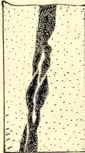
Fig. 5.—Section of a segregation band of chromitiferous olivine rock in the saxonite of Varnasfjeld. (Vogt.) Length of lode 40 to 50 meters; thickness 0.1-0.8 meters.
