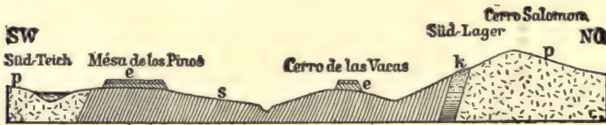
Fig. 50.—Profile through a part of the Rio Tinto ore field. (A. Phillips.) s, clay slate; p, porphyry; k, copper ore bed; e, Pleistocene iron ores.
