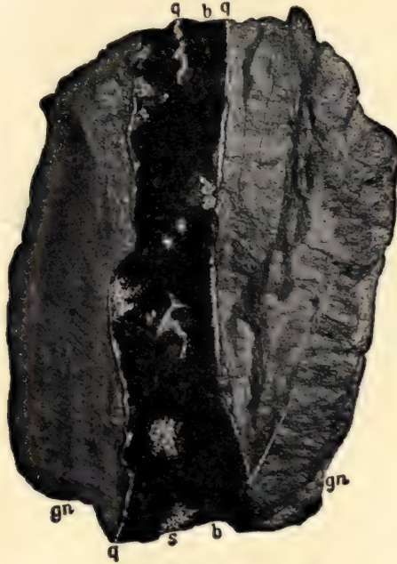
Fig. 128.—View of the Rudolf Stehende (pyritous lead ore formation) with dominant massive structure. (From nature.) gr, decomposed gray gneiss; q, quartz; b, argentiferous galena; s, pyrite.
