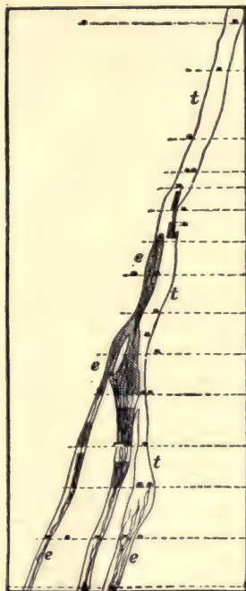
Fig. 157.—Cross-section through the main veins of the Bergmannstrost mine, 70 m. east of the Marien shaft. (Zirkler.)
