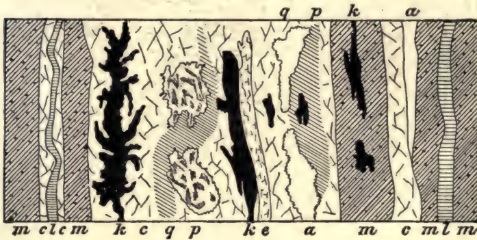
Fig. 153.—Cross-section through Cliff lode. (H. Credner.)
