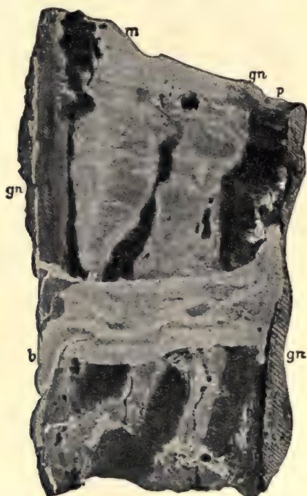
Fig. 127.—View of the Komet Stehende (Carbonspathic lead formation) with a cross stringer.
