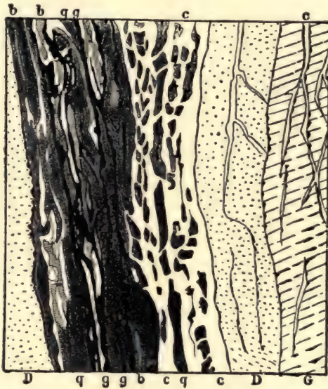
Fig. 161.—The Adalbert main vein at Pribram. (J. Zadrazil, reproduced by J. Schmid.) G, graywacke; D, diorite; q, quartz; c, calcspar; g, galena; b, zinc-blende.
