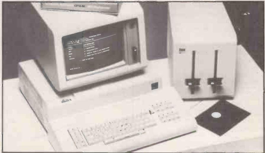
The IBM format is industry standard for 8in. discs — but the PC has 5.25in. drives.
