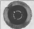
Fig 1. A daisy wheel and the rest of small size print from it
