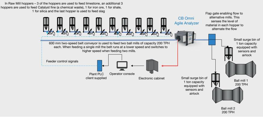
Figure 9: Depiction of an automated, integrated solution that is both efficient and sustainable
