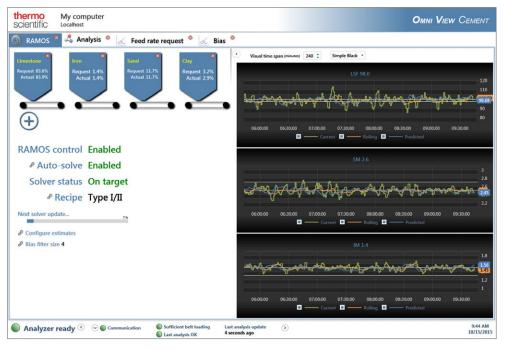
Figure 8: RAMOS software manipulating the feed rate of four different materials
