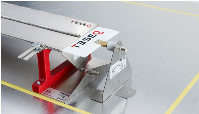
Fig. 4: connection of termination bracket (connecting adapter)
