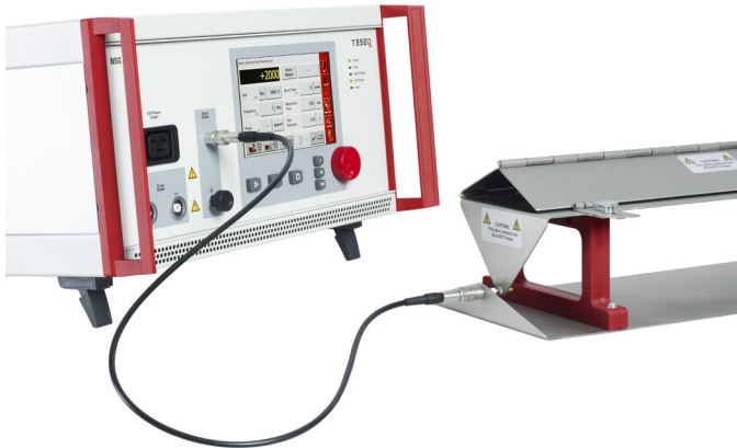
Fig. 3: CDN 3425 connected to the EFT output of a NSG 3040 generator
