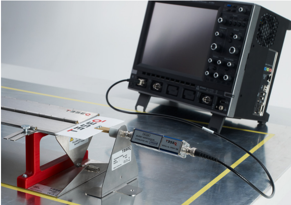
Fig. 5: CAS 3025 (INA 265A – 50 \Omega terminator/attenuator) and oscilloscope connected to termination bracket.
