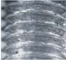
Flaky surface due to insufficient lubrication; solution: Lubrication grooves
