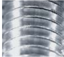
Smooth surface due to excellent lubrication
