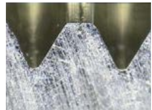
Thread profile made with a special former
