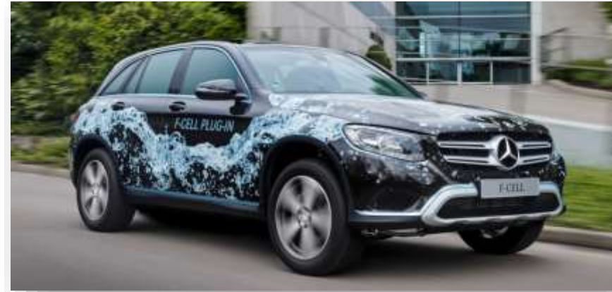
Mercedes GLC, fuel cell with plug-in-battery, 500 km range (50 km by battery)
