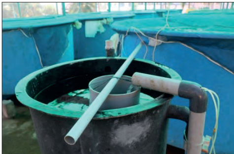
Fig. 32. Copepod nauplii harvesting tank used in Visakhapatnam Centre of CMFRI
