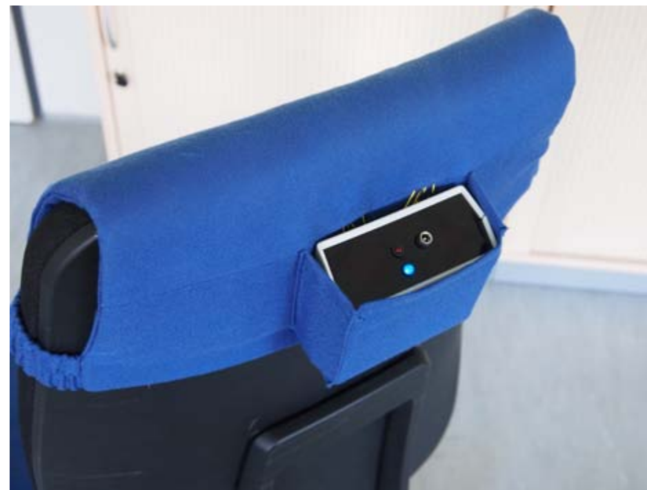
Controller-box - switches have meanwhile be replaced by less error prone hidden magnetic contacts.
