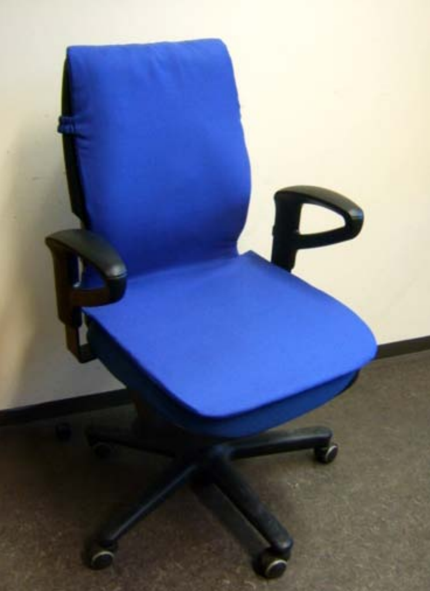
SonicChair Sensor lay-on attached to a standard office chair.
