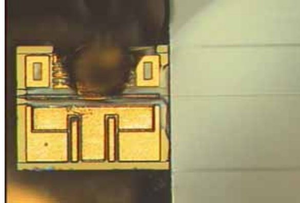
Fig. 4: A LD chip is butt coupled to a polymer waveguide.
