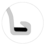
Interlock with bitumen
