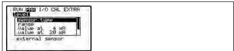
Fig. 9-26 Example in case of external level sensor
