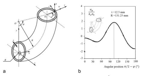
Fig. 1. a: Geometrical dimensions of a curved pipe. b non-dimensional hoop stress  $\frac{\sigma_{\varphi}}{k_{\tau\sigma_0}}$  versus angular position
