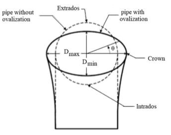
Fig. 2. Definition of minimum and maximum diameter for the flattening parameter.
